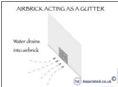
Air brick acting as gutter
