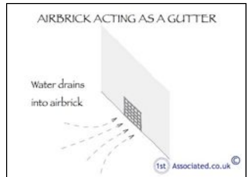
Air brick, acting as a gutter
