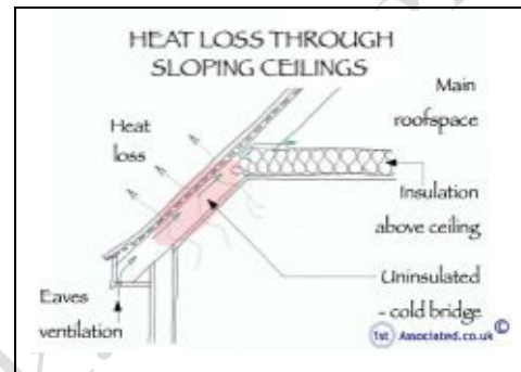
Heat is lost where ceilings are sloping and partly in the roof
