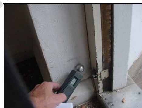
Testing for rising damp
