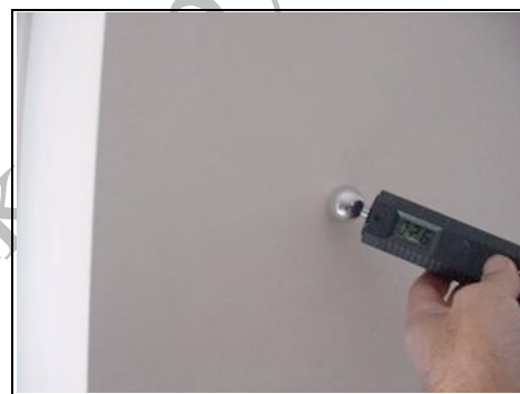
Testing for lateral dampness
