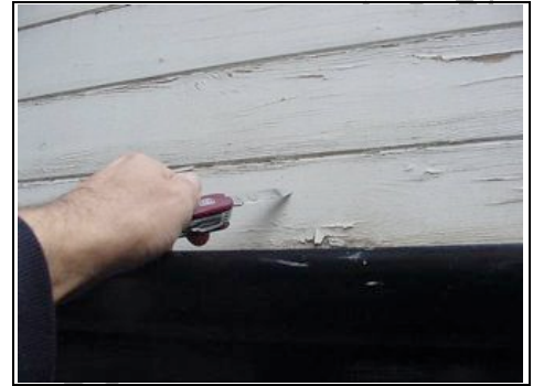
Knife test to fascia board
