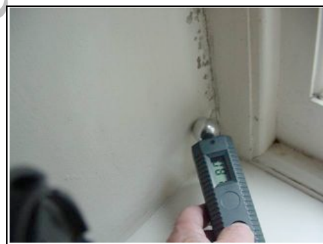
High damp readings in the annexe
