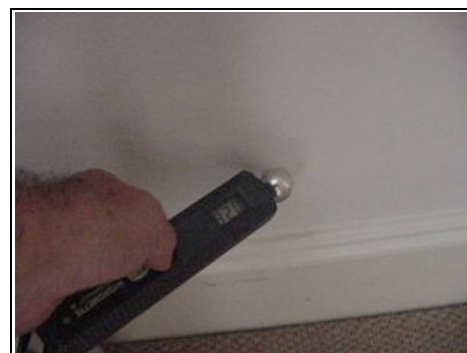
Testing for rising damp
