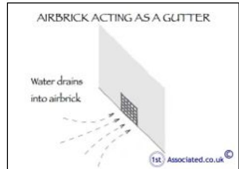
Air brick acting as a gutter
