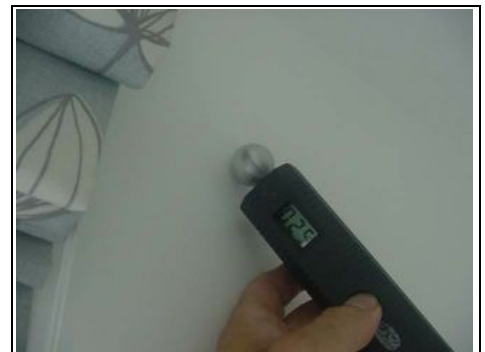
Checking that the flat roof is not leaking allowing dampness in
