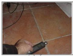
Checking dampness to floor on rear lower ground floor right side under the stairs
