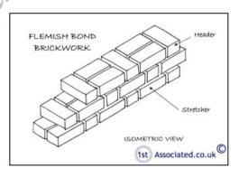
Flemish bond brickwork
