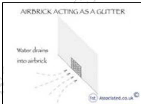
Air brick acting as a gutter
