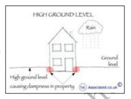
**ACTION REQUIRED**: Lower ground level and add French drain.
