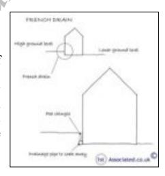
The French drain acts as an area where water soaks away quickly. We often recommend them close to building, but not next to the building, as this helps reduce the ground level and/or take any water that is directed at that area away. For example, where a patio has been put in place which aims any rainwater at part of the wall. As mentioned, whilst a French drain is a D.I.Y. job, it does need some understanding of how it works.
