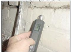
Surprisingly dry in basement, expected readings of 60 plus, obtained reading of 42
