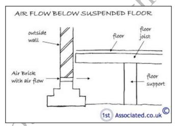
Air bricks are essential to have a Suspethrough flow of air as this helps to reduce the chances of wet rot, dry rot and woodworm.
