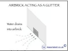
Air brick acting as gutter
