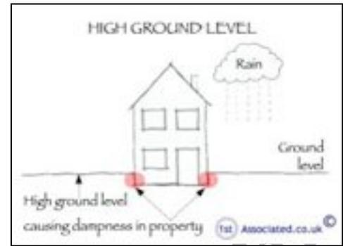
**ACTION REQUIRED:** Lower ground level and add French drain.
