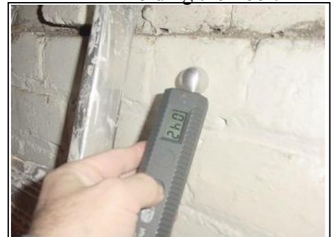
Surprisingly dry in basement, expected readings of 60 plus, obtained reading of 42
